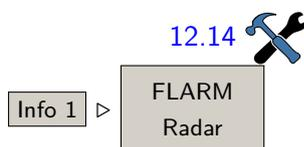
Once FLARM has reported traffic and the small radar-style view of the FLARM traffic gets activated you can tap on the FLARM radar to enlarge the view to fullscreen size. The fullscreen FLARM display offers all available information about the FLARM traffic and depending on the setup it closes by itself, when all traffic has gone.
