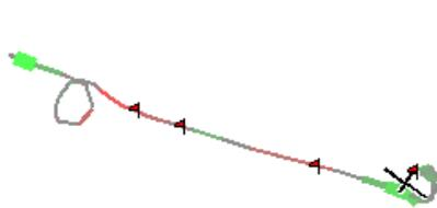
If Vega or an intelligent variometer is connected with Netto output, the Netto vario value is used; hence the colours and thickness of the trail indicates the air-mass vertical movement rather than the glider's vertical movement.
