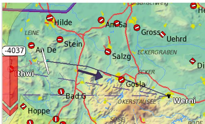
Routes take into account the glider polar performance and are calculated to be optimal in the sense of minimum time. By default, route calculation is disabled, and can be enabled for terrain only or terrain and airspace avoidance.
