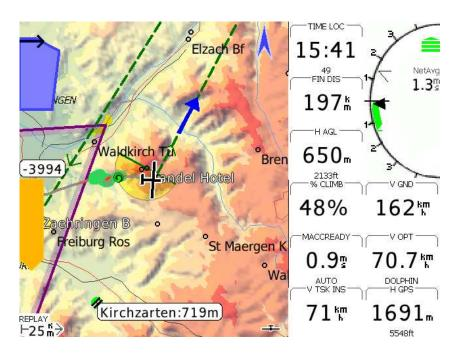
Figure 3.1: Typical XCSoar main screen layout
