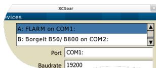
COM ports 0 to 10 may be used, including a TCP/IP connection. Which COM port is appropriate for you depends on what brand of PDA you use, and the communications medium (serial cable, Bluetooth, virtual COM port, SD card or CF based GPS, internal GPS). Detailing the various options for different devices is beyond the scope of this document. If you have trouble identifying which COM port to set, please refer to the XCSoar website and mailing lists.
