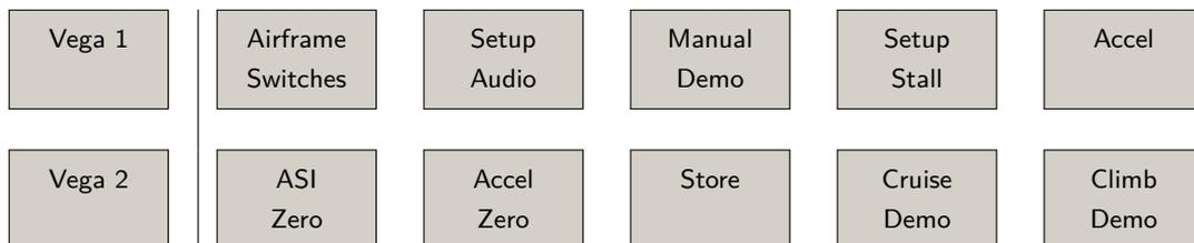
The functions in this sub-menu require the Vega intelligent variometer. The menu can only be accessed if 'Vega' is selected as the connected device.
