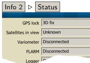
The system status dialogue is used primarily as a systems check, to see how the glide computer and the connected devices are performing. This is accessed via the menu and then selecting the tabular **System**.
