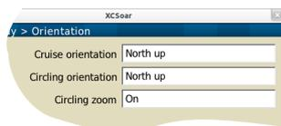
**Heading up:** The moving map display will be rotated so the glider's heading is oriented up.
