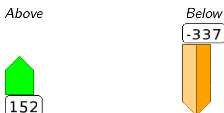
The scale of the final glide bar is  $\pm 500$  meters.
