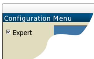
The main configuration dialogue (Setup System) can be run in Basic or Expert user level, via a selectable field on the left of the dialogue. When in Basic mode, many of the less commonly used and advanced configuration settings are hidden. In the descriptions below, all of the parameters marked with an asterisk are only visible in expert user level.
