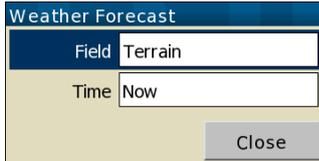
The Field setting determines which data field is displayed on the map. The Time setting determines at which forecast time the data field will be displayed. Upon entering the weather dialogue, the Time setting is advanced to the next nearest forecast time available in the RASP file. When a field is not available in the RASP file, the background is left blank.
