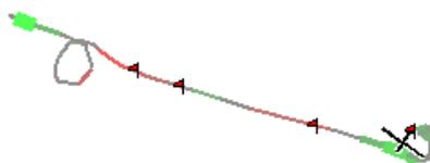
If Vega or an intelligent variometer is connected with Netto output, the Netto vario value is used; hence the colours and thickness of the trail indicates the air-mass vertical movement rather than the glider's vertical movement.
