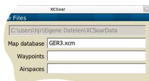
The first time that XCSoar is run, it does not automatically load the data files that you placed in the XCSoarData directory. To tell XCSoar which files to load, double click/tap the map (the large, blank white part with the glider symbol in the center), choose the menu **Config 2** (click/tap it twice), then select the item **System**. The Configuration screen should be displayed: The first page allows you
