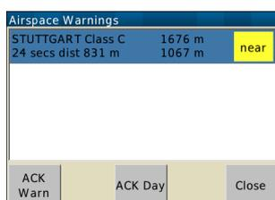
At all times XCSoar monitors the aircraft relative to all airspace and maintains warning levels for each. The airspace warnings are still filtered according to the airspace filter preferences; such that certain categories of airspace may be effectively disabled. The sequence of events when entering an airspace results typically in two warnings: when near (level 1), and when inside (level 2).
