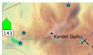
While climbing in thermals, a marker is automatically generated showing the thermal location on screen. The positions of the last 20 thermals are stored until the end of the flight. This thermal history is accessible through the map element functions in the same way as markers or waypoints.
