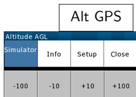
This is the altitude above mean sea level reported by the GPS. (Touch-screen/PC only) In simulation mode this value is adjustable with the up/down arrow keys. The right/left arrow keys also cause the glider to turn.<sup>1</sup>
