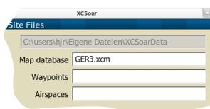
Airspace files define Special Use Airspace. Up to two files may be specified, the first for the main SUA file, and the second is intended for use with NOTAM airspace, and is referred to as the additional airspace file.
