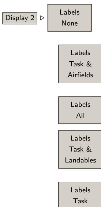
The screen can be de-cluttered, turning off the display of all waypoint labels by toggling the 'Labels' menu.
