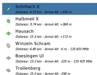
Alternates are maintained throughout the flight, reflecting good air-anship by always keeping an eye on possible alternates. Six landing options are maintained. They are filtered by the configured "alternates mode" criteria (Simple, Task, or Home). Choosing Task or Home puts some bias on the presentation of alternates to the heading, you were taking whilst still task oriented.
