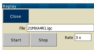
Flight logs in the IGC format generated by XCSOar or other loggers can be replayed. The logger replay dialogue can be accessed via the menu:
