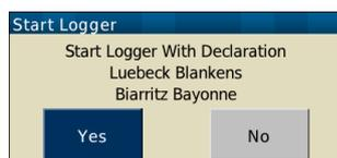
The logger can be turned on and off automatically or manually. For para-glider XCSoar provides the option to only start the logger automatically. Thus a very slow and close to the terrain flight won't automatically stop logging the flight. If you choose the auto start only logger you have to stop the logger manually. To turn the logger on (or off) manually, select from the menu:
