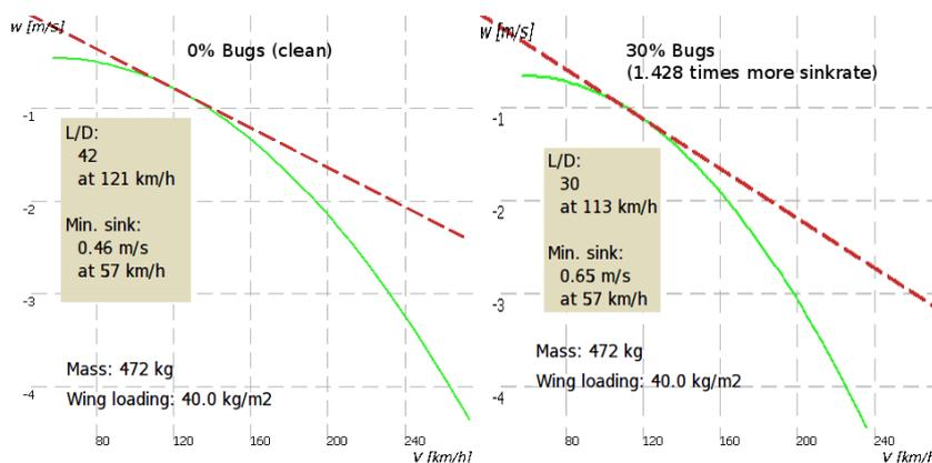
Knowing all this, a meaningful setting for a worst-case bug polluted wing could scale down the polar by 30%. Some experimentation may be required to determine appropriate settings for bugs, because the performance degradation experienced by different glider types may be different.
