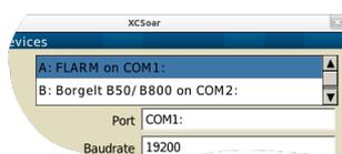
The Devices page is used to specify the ports used to communicate with the GPS and other serial devices. The default settings are COM1 and 4800 bits per second. When connected to the Vega intelligent variometer, the settings should be COM1 and 38400.
