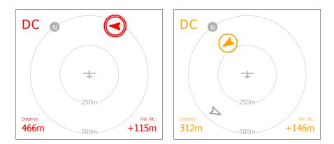
The three screenshots are taken in a sequence and demonstrate a typical near pass of e.g. two FLARM equipped gliders. The extra information is colour-coded in the already mentioned way. In the four corners of the radar screen is additional info to the selected target displayed:
