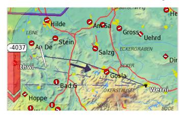
Routes take into account the glider polar performance and are calculated to be optimal in the sense of minimum time. By default, route
