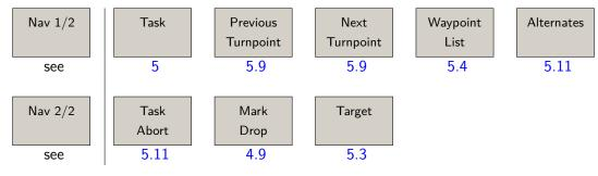
You should not start using XCSoar without knowing about the 'Alternates' feature. Any 'Task' related item in the navigation menu is used for planned cross country flight and certainly the second step.
