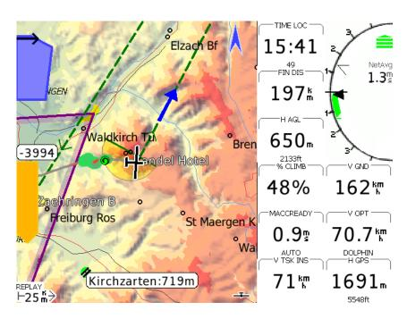
Figure 3.1: Typical XCSoar main screen layout
