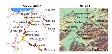
If the terrain data is not available (or terrain display is turned off), the background colour of the map window is white. All terrain below mean sea level is coloured blue. If you are flying outside the terrain region, the background colour will be white.
