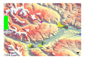
Turning : If turning reach is enabled, then the reach shows the greatest area the glider can reach in all directions, even allowing turns
