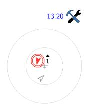
The FLARM targets on the map are drawn as red coloured arrow heads to indicate the direction the FLARM target is heading, as well as the collision risk. Note that these arrow heads are oriented according to the display orientation. For example, if the orientation is trackup, then the arrows show the relative track bearing of the target to the aircraft. If the orientation is north-up, then the arrows show the absolute track bearing of the target.
