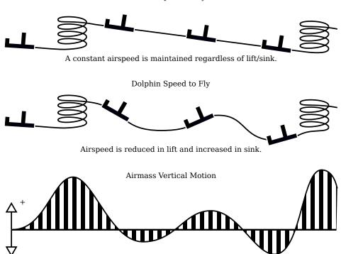
A configuration option 'Block speed to fly' (see Section 12.11) can be used to specify whether dolphin or block speed to fly is used. The infobox 'V Opt' shows the optimum speed according to whichever mode is selected. When connected to the Vega intelligent variometer, the speed command sounds are based on this optimum speed value.
