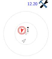
To remedy this situation, when FLARM traffic is received, XCSoar shows a small radar-style view of the FLARM traffic from the perspective of the aircraft. The FLARM traffic is displayed in identical style, except that the threatening traffic is emphasized with one or two red circles around the arrow head icon. The display corner used for the small radar view can be configured.
