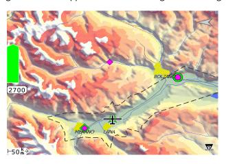
Turning: If turning reach is enabled, then the reach shows the greatest area the glider can reach in all directions, even allowing turns
