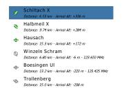
Alternates are maintained throughout the flight, reflecting good airmenship by always keeping an eye on possible alternates. Six landing options are maintained. They are filtered by the configured "alternates mode" criteria (Simple, Task, or Home). Choosing Task or Home puts some bias on the presentation of alternates to the heading, you were taking whilst still task oriented.
