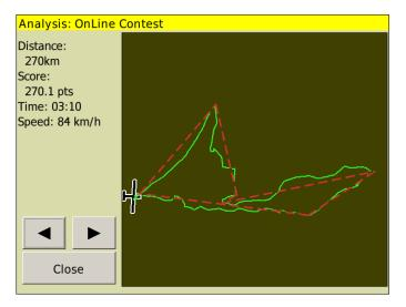
When flying for contests, either AAT or non-AAT tasks may still be used to manage the flight navigation. During flight, the computer will optimise the current flight with respect to the selected contest rules.
