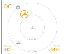
The three screenshots are taken in a sequence and demonstrate a typical near pass of e.g. two FLARM equipped gliders. The extra information is colour-coded in the already mentioned way. In the four corners of the radar screen is additional info to the selected target displayed:
