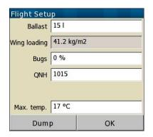
The 'bugs' setting determines the amount the polar is degraded due to contamination during a long flight. A 'bugs' setting of 0% will cause the software to use the clean polar. A 'bugs' setting of 50% will degrade the polar and effectively double the sink rate for a given airspeed.
