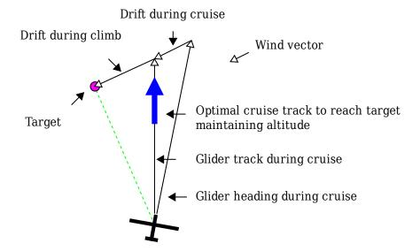
The optimal cruise track is displayed on the map area as a large blue arrow, and it recommends the glider steers so that the glider's track is lined up with the blue arrow during cruise. For example, if the display is oriented 'Track-Up', then steer so the blue arrow points directly up.
