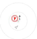
To remedy this situation, when FLARM traffic is received, XCSoar shows a small radar-style view of the FLARM traffic from the perspective of the aircraft. The FLARM traffic is displayed in identical style, except that the threatening traffic is emphasized with one or two red circles around the arrow head icon. The display corner used for the small radar view can be configured.
