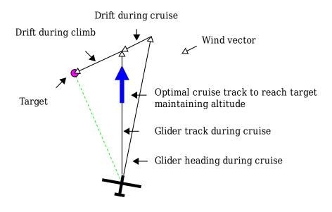
The optimal cruise track is displayed on the map area as a large blue arrow, and it recommends the glider steers so that the glider's track is lined up with the blue arrow during cruise. For example, if the display is oriented 'Track-Up', then steer so the blue arrow points directly up.
