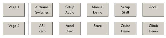
The functions in this sub-menu require the Vega intelligent variometer. The menu can only be accessed if 'Vega' is selected as the connected device.
