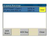
At all times XCSoar monitors the aircraft relative to all airspace and maintains warning levels for each. The airspace warnings are still filtered according to the airspace filter preferences; such that certain categories of airspace may be effectively disabled. The sequence of events when entering an airspace results typically in two warnings: when near (level 1), and when inside (level 2).
