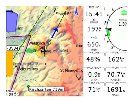
Figure 3.1: Typical XCSoar main screen layout
