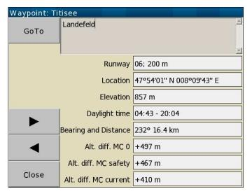
As mentioned above, the Waypoint info dialogue also shows three forms of altitude difference (additional altitude required to reach the waypoint at the safety height) for the corresponding waypoint:
