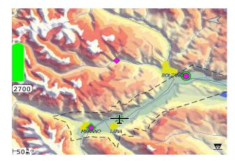
Turning: If turning reach is enabled, then the reach shows the greatest area the glider can reach in all directions, even allowing turns around obstructions. The reach area appears as a closed ring around the glider but may also include holes indicating mountain peaks that the glider cannot reach without further climb.
