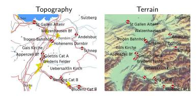
If the terrain data is not available (or terrain display is turned off), the background colour of the map window is white. All terrain below mean sea level is coloured blue. If you are flying outside the terrain region, the background colour will be white.
