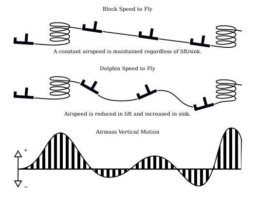
A configuration option 'Block speed to fly' (see Section 12.11) can be used to specify whether dolphin or block speed to fly is used. The infobox 'V Opt' shows the optimum speed according to whichever mode is selected. When connected to the Vega intelligent variometer, the speed command sounds are based on this optimum speed value.
