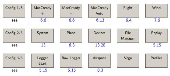
The configuration menu is typically part of the ground interaction with XCSoar. You are not expected to spend much time in-flight with tweaking the configuration, except you manually adjust wind or MacCready settings. The 'Vega' item gives control over the Vega intelligent variometer. This comprises a sub-menu.
