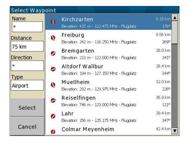
The list can be scrolled if there is more than one screen full of matching waypoints. To scroll through the list, simply drag with the finger, or move to the bottom (or top) of the list with the cursor.
