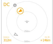
The three screenshots are taken in a sequence and demonstrate a typical near pass of e.g. two FLARM equipped gliders. The extra information is colour-coded in the already mentioned way. In the four corners of the radar screen is additional info to the selected target displayed:
