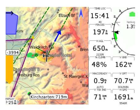
Figure 3.1: Typical XCSoar main screen layout
