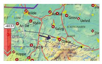
Routes take into account the glider polar performance and are calculated to be optimal in the sense of minimum time. By default, route calculation is disabled, and can be enabled for terrain only or terrain and airspace avoidance.
