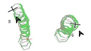
Enabling trail drift compensation is performed through the configuration settings. The compensation is only performed whilst in circling mode; the display of the trail in cruise mode is unaffected. This can also be performed from the wind settings dialogue.
