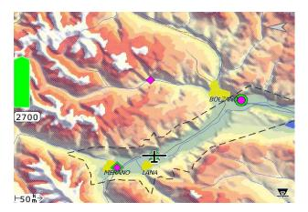
Turning : If turning reach is enabled, then the reach shows the greatest area the glider can reach in all directions, even allowing turns around obstructions.<sup>4</sup> The reach area appears as a closed ring around the glider but may also include holes indicating mountain peaks that the glider cannot reach without further climb.
