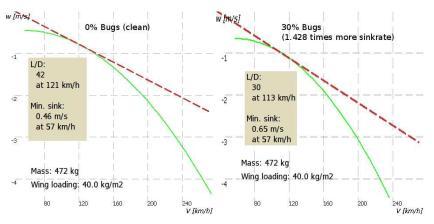
Knowing all this, a meaningful setting for a worst-case bug polluted wing could scale down the polar by 30%. Some experimentation may be required to determine appropriate settings for bugs, because the performance degradation experienced by different glider types may be different.
