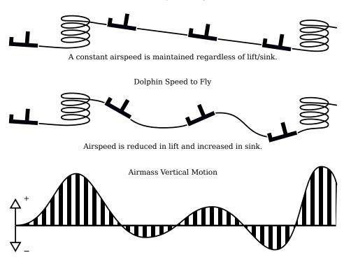
A configuration option 'Block speed to fly' (see Section 13.11) can be used to specify whether dolphin or block speed to fly is used. The infobox 'V Opt' shows the optimum speed according to whichever mode is selected. When connected to the Vega intelligent variometer, the speed command sounds are based on this optimum speed value.
