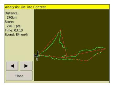
When flying for contests, either AAT or non-AAT tasks may still be used to manage the flight navigation. During flight, the computer will optimise the current flight with respect to the selected contest rules.
