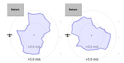
The two screen-shots are taken in a few seconds sequence to demonstrate the practical usage of the rotating climb diagram. A simple recipe to optimise the climb rate according to the assistant would be to follow these two steps repeatedly:
