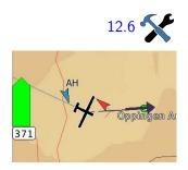
The FLARM targets on the map are drawn as red coloured arrow heads to indicate the direction the FLARM target is heading, as well as the collision risk. Note that these arrow heads are oriented according to the display orientation. For example, if the orientation is track-up, then the arrows show the relative track bearing of the target to the aircraft. If the orientation is north-up, then the arrows show the absolute track bearing of the target.
