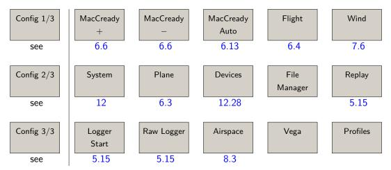
The configuration menu is typically part of the ground interaction with XCSoar. You are not expected to spend much time in-flight with tweaking the configuration, except you manually adjust wind or MacCready settings. The 'Vega' item gives control over the Vega intelligent variometer. This comprises a sub-menu.
