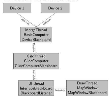
The device driver parses input received from its device into its own NMEAInfo instance inside DeviceBlackboard (i.e. per\_device\_data). Then it wakes up the MergeThread to merge the new data into the central NMEAInfo instance. The MergeThread hosts the
