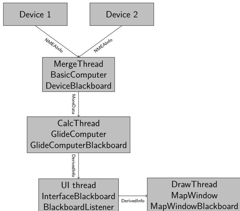
The device driver parses input received from its device into its own `NMEAInfo` instance inside `DeviceBlackboard` (i.e. `per_device_data`). Then it wakes up the `MergeThread` to merge the new data into the central `NMEAInfo` instance. The `MergeThread` hosts the
