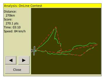
When flying OLC, either AAT or non-AAT tasks may still be used to manage the flight navigation. During flight, the computer will optimise the current flight with respect to the selected OLC rules.
