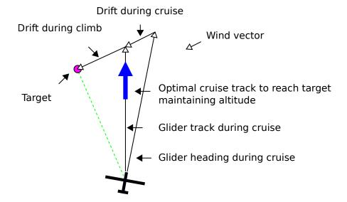
The optimal cruise track is displayed on the map area as a large blue arrow, and it recommends the glider steers so that the glider's track is lined up with the blue arrow during cruise. For example, if the display is oriented 'Track-Up', then steer so the blue arrow points directly up.
