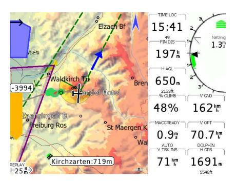
Figure 3.1: Typical XCSoar main screen layout
