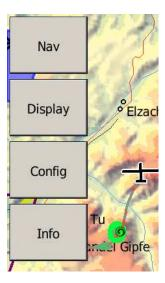
The menu is organised into four different groups of functions, usually in the form of a hierarchy. The specific menu layout depends on the hardware button configurations and platform, and may also be customised by the user.
