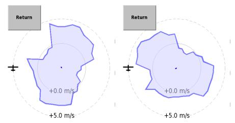
The two screen-shots are taken in a few seconds sequence to demonstrate the practical usage of the rotating climb diagram. A simple recipe to optimise the climb rate according to the assistant would be to follow these two steps repeatedly:
