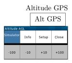
This is the altitude above mean sea level reported by the GPS. (Touch-screen/PC only) In simulation mode this value is adjustable with the up/down arrow keys. The right/left arrow keys also cause the glider to turn.<sup>1</sup>
