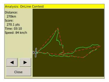
When flying OLC, either AAT or non-AAT tasks may still be used to manage the flight navigation. During flight, the computer will optimise the current flight with respect to the selected OLC rules.
