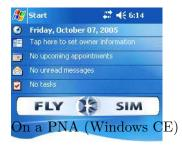
Download the program file XCSoar.exe to a SD card. You can launch it with the File Explorer. Another method to install XCSoar on a PDA is the CAB file. Download it to the SD card. Use the File Explorer to install it. After the installation, the XCSoar 'FLY' and 'SIM' launcher icons will be visible on the Today screen.
