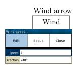
Wind vector estimated by XCSoar. Manual adjustment is possible with the connected InfoBox dialogue. Pressing the up/down cursor keys to cycle through settings, adjust the values with left/right cursor keys.
