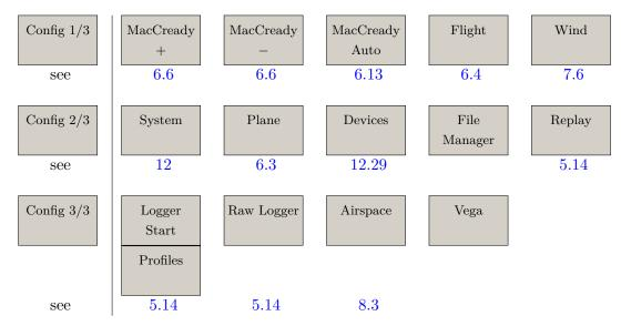
The configuration menu is typically part of the ground interaction with XCSoar. You are not expected to spend much time in-flight with tweaking the configuration, except you manually adjust wind or MacCready settings. The 'Vega' item gives control over the Vega intelligent variometer. This comprises a sub-menu.
