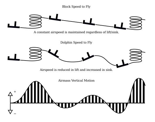
A configuration option 'Block speed to fly' (see Section 13.11) can be used to specify whether dolphin or block speed to fly is used. The infobox 'V Opt' shows the optimum speed according to whichever mode is selected. When connected to the Vega intelligent variometer, the speed command sounds are based on this optimum speed value.
