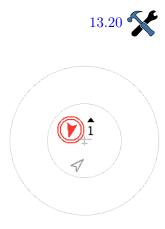
To remedy this situation, when FLARM traffic is received, XC-Soar shows a small radar-style view of the FLARM traffic from the perspective of the aircraft. The FLARM traffic is displayed in identical style, except that the threatening traffic is emphasized with one or two red circles around the arrow head icon. The display corner used for the small radar view can be configured.
