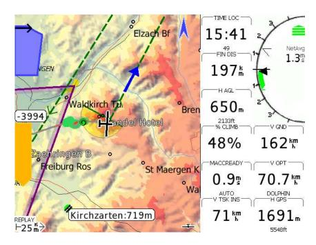
Figure 3.1: Typical XCSoar main screen layout
