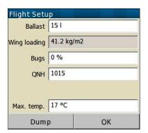
The 'bugs' setting determines the amount the polar is degraded due to contamination during a long flight. A 'bugs' setting of 0% will cause the software to use the clean polar. A 'bugs' setting of 50% will degrade the polar and effectively doubling the sink rate for a given airspeed.
