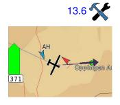
The FLARM targets on the map are drawn as red coloured arrow heads to indicate the direction the FLARM target is heading, as well as the collision risk. Note that these arrow heads are oriented according to the display orientation. For example, if the orientation is track-up, then the arrows show the relative track bearing of the target to the aircraft. If the orientation is north-up, then the arrows show the absolute track bearing of the target.
