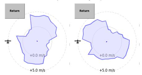
The to screen-shots are taken in a few seconds sequence to demonstrate the practical usage of the rotating climb diagram. A simple recipe to optimise the climb rate according to the assistant would be to follow these two steps repeatedly:
