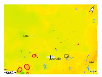
BL wind spd: The speed and direction of the vector-averaged wind in the BL. This prediction can be misleading if there is a large change in wind direction through the BL.
