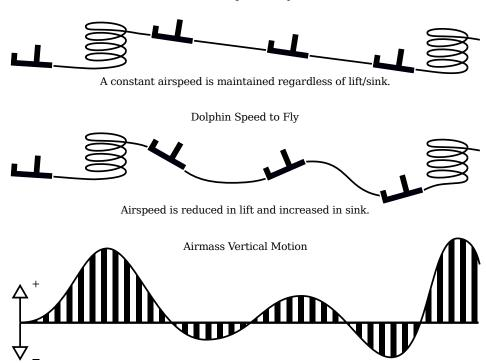
A configuration option 'Block speed to fly' (see Section 12.10) can be used to specify whether dolphin or block speed to fly is used. The infobox 'V Opt' shows the optimum speed according to whichever mode is selected. When connected to the Vega intelligent variometer, the speed command sounds are based on this optimum speed value.
