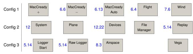
The configuration menu is typically part of the ground interaction with XCSoar. You are not expected to spend much time in-flight with tweaking the configuration, except you manually adjust wind or MacCready settings. The 'Vega' item gives control over the Vega intelligent variometer. This comprises a sub-menu.
