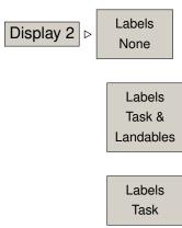
The screen can be de-cluttered, turning off the display of topography labels and non-task waypoint labels by toggling the 'Labels' menu.
