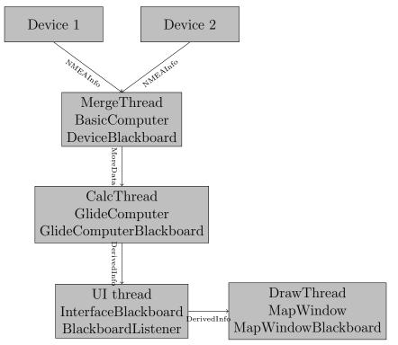
The device driver parses input received from its device into its own NMEAInfo instance inside DeviceBlackboard (i.e. per\_device\_data). Then it wakes up the MergeThread to merge the new data into the central NMEAInfo instance. The MergeThread hosts the BasicComputer which attempts to calculate missing data (for example, derives vario from GPS altitude).
