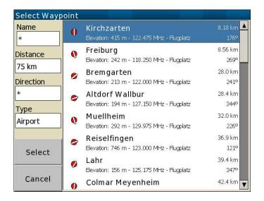
The list can be scrolled if there is more than one screen full of matching waypoints. To scroll through the list, simply drag with the finger, or move to the bottom (or top) of the list with the cursor.
