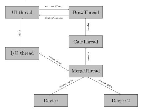
The UI thread is the main thread. It starts the other threads and is responsible for the UI event loop. No other thread is allowed to manipulate windows. The UI thread has a timer which does regular house keeping twice per second (Process-Timer.cpp).
