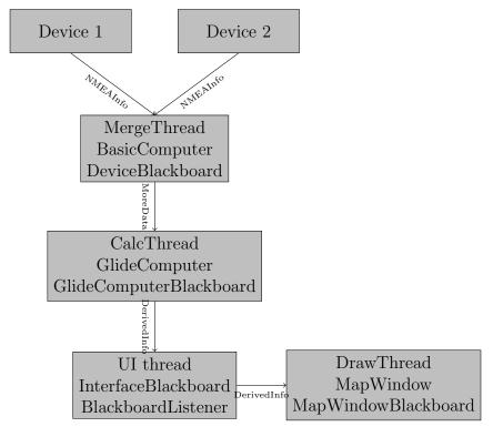
The device driver parses input received from its device into its own NMEAInfo instance inside DeviceBlackboard (i.e. per\_device\_data). Then it wakes up the MergeThread to merge the new data into
