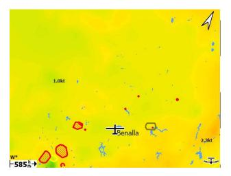
BL wind spd: The speed and direction of the vector-averaged wind in the BL. This prediction can be misleading if there is a large change in wind direction through the BL.
