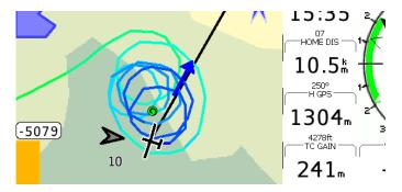
The thermal locator marks the location of the last 20 thermals on the map with the thermal symbol during cruise.
