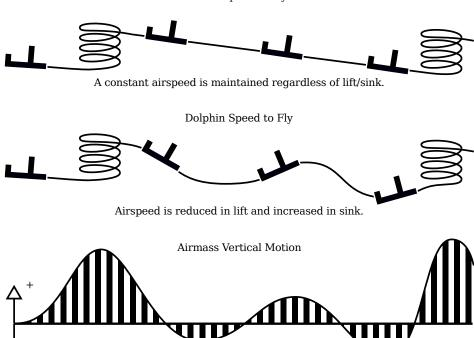
A configuration option 'Block speed to fly' (see Section 12.10) can be used to specify whether dolphin or block speed to fly is used. The infobox 'V Opt' shows the optimum speed according to whichever mode is selected. When connected to the Vega intelligent variometer, the speed command sounds are based on this optimum speed value.
