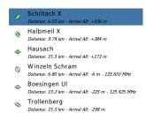
Alternates are maintained throughout the flight. In contrast to the abort mode options is the idea to have continously an eye on possible alternates. Six landing options are maintained. They are filtered by the configured 'alternates mode' criteria (Simple, Task, or Home). One of those criterias should fit to your personal preference.
