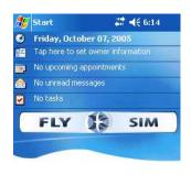
on a PDA is the CAB file. Download it to the SD card. Use the File Explorer to install it. After the installation, the XCSoar 'FLY' and 'SIM' launcher icons will be visible on the Today screen.
