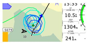
The thermal locator marks the location of the last 20 thermals on the map with the thermal symbol during cruise.
