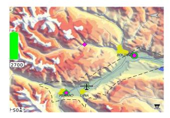
Turning : If turning reach is enabled, then the reach shows the greatest area the glider can reach in all directions, even allowing turns around obstructions.<sup>3</sup> The reach area appears as a closed ring around the glider but may also include holes indicating mountain peaks that the glider cannot reach without further climb.
