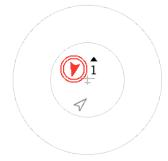
To remedy this situation, when FLARM traffic is received, XCSoar shows a small radar-style view of the FLARM traffic from the perspective of the aircraft. The FLARM traffic is displayed in identical style, except that the threatening traffic is emphasized with one or two red circles around the arrow head icon. The display corner used for the small radar view can be configured.
