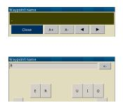
To enter text in 'high score style', use the A+/A- buttons to adjust the character under the cursor (underlined character). Clicking the and > buttons move the cursor left/right.
