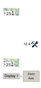
The map scale is displayed in the lower left corner of the moving map display. The indicated distance is measured from the left to the right boarder of the map display.
