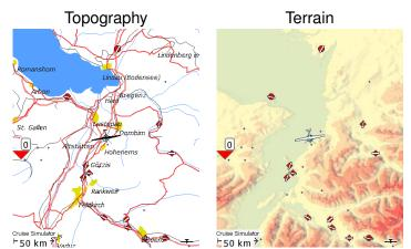
If the terrain data is not available (or terrain display is turned off), the background colour of the map window is white. All terrain below mean sea level is coloured blue. If you are flying outside the terrain region, the background colour will be white.
