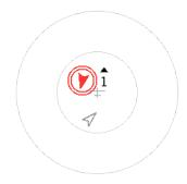
To remedy this situation, when FLARM traffic is received, XCSoar shows a small radar-style view of the FLARM traffic from the perspective of the aircraft. The FLARM traffic is displayed in identical style, except that the threatening traffic is emphasized with one or two red circles around the arrow head icon. The display corner used for the small radar view can be configured.
