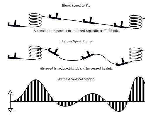
A configuration option 'Block speed to fly' (see Section 12.10) can be used to specify whether dolphin or block speed to fly is used. The infobox 'V Opt' shows the optimum speed according to whichever mode is selected. When connected to the Vega intelligent variometer, the speed command sounds are based on this optimum speed value.
