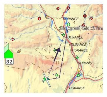
Routes take into account the glider polar performance and are calculated to be optimal in the sense of minimum time. By default, route calculation is disabled, and can be enabled for terrain only or terrain and airspace avoidance.
